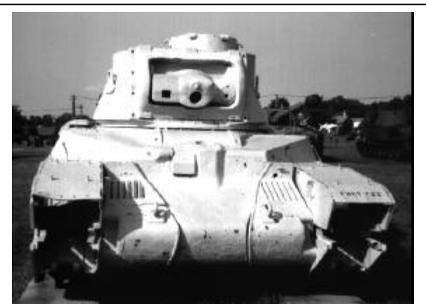
Nose-on view of the British A12 Matilda Infantry Tank Mark II parked at Aberdeen. Note the many angles making up the front of the tank. In the entries in this book, I used the armour thicknesses and angles I felt provided an aggregate value for the surface area noted.
